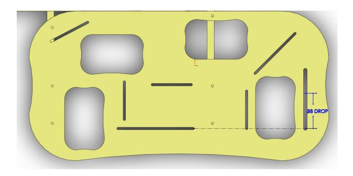
Part #11 is optional, but can be used to support the Seatstays and Chainstays. It can be bolted to the backplate and adjusted to cradle both CS and SS if needed. It can be seen in the entire assembly image below.
