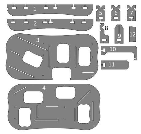
1. Left Rib 2. Right Rib 3. Upper Backplate 4. Lower Backplate 5. V Block 25.4 6. V Block 28.6 7. V Block 31.7 8. V Block Multi Size 9. HT Bracket 10. Dropout Holder 11. CS/SS Support 12. Dropout Ruler (130mm / 135mm)
