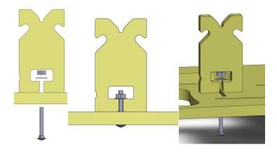
You may want to secure tubes to v-blocks. This is done using steel or copper wire, wrapping it under the hooks on the v block and over the tube and twisting with a pliers. This will pull the tube against the surface of the V and hold it securely. Bend exposed wire tails out of the way to avoid them scratching or poking you.
