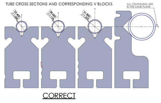
Note each V block shown has dimples on the lower left side. A single dimple indicates the V block is made for a 25.4mm diameter tube, two dimples is for a 28.6mm diameter tube, and three dimples is for a 31.7mm diameter tube. These are very common tube sizes and should work for most frames. But what if I'm not using those sizes??? You're in luck because we also have included a universal V block that can hold a tube of any diameter in the same plane (shown as right most V block in picture above).
